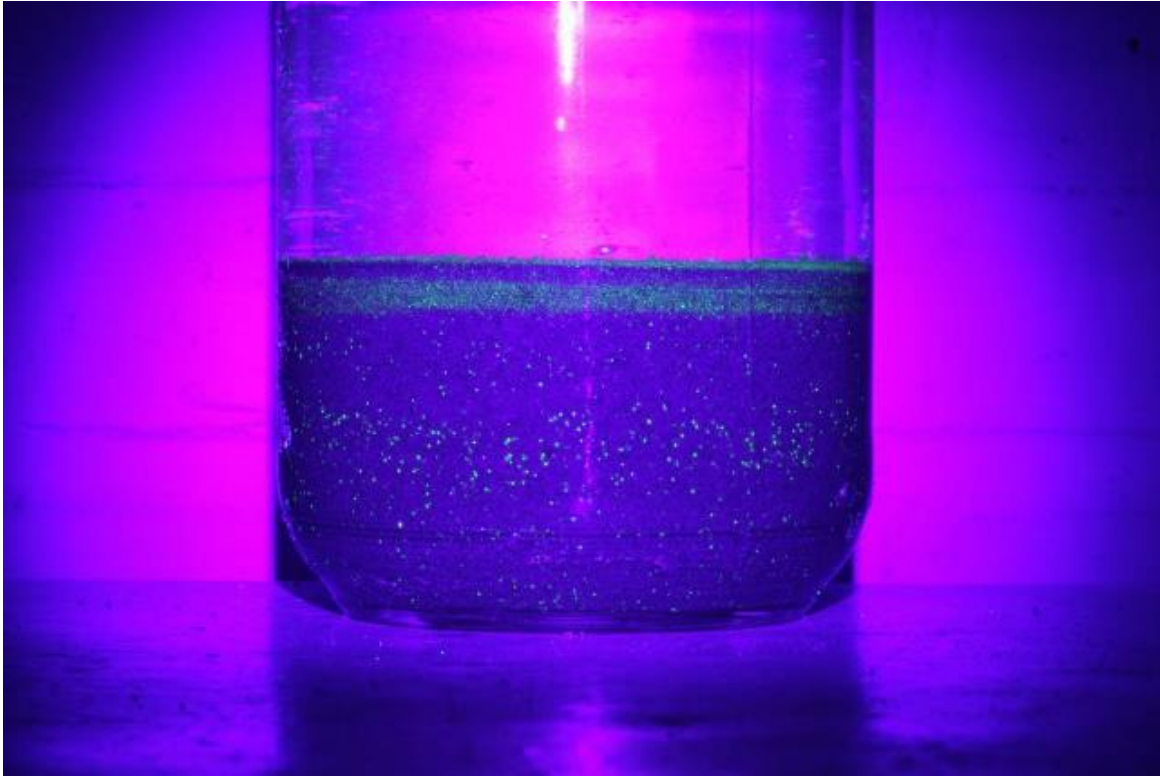
Figure 3.19 Example of tracer sediment recovered from the seabed. The sample is illuminated under ultraviolet light, which causes the tracer particles to appear as green dots, and native sediment as the darker purple matrix surrounding them.
