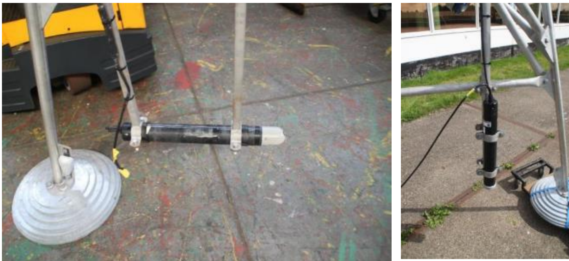
Figure 3.4 Downward looking ADCP-HRs with sideward (left) and downward (right) head configuration.
