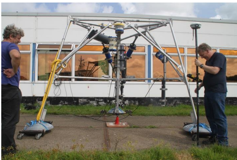
Figure C.2 Compass calibration procedure. The frame was rotated around the centre pole.
